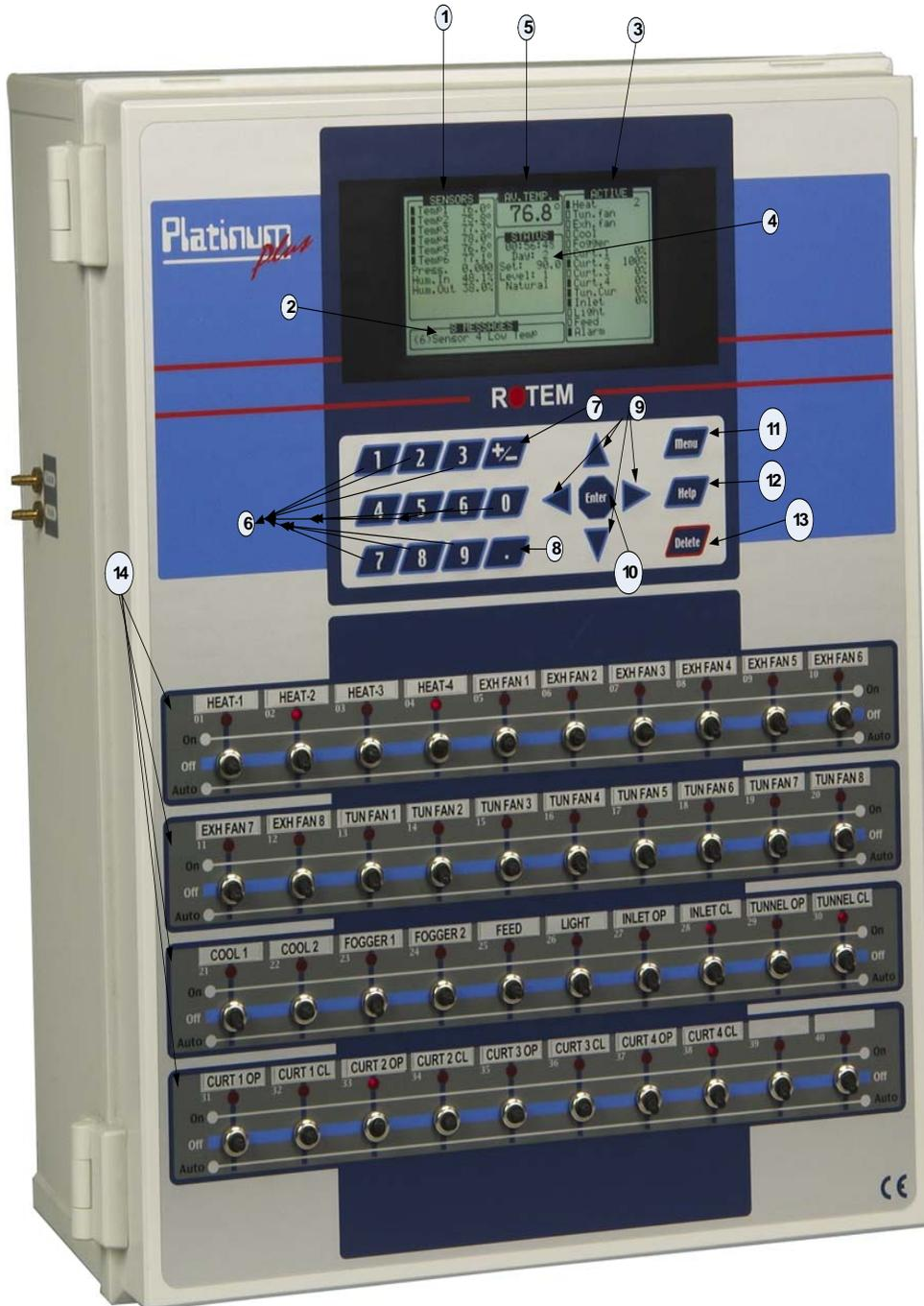
**Fig. 2: Platinum Plus's front panel**
