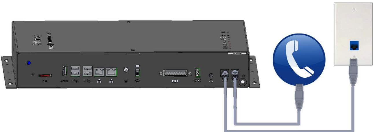
*NOTE The telephone line-modem output connection wiring must provide double insulation. Use minimum 26 AWG wiring or larger for telephone line connection.*
