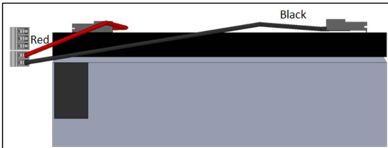
8. Remove the battery and put the new battery in place.
